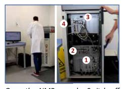
Open the NMR console. Switch off all units from bottom to top (1-3). Give each unit time to shut down completely to avoid any system errors. Then turn off the console power (4).
