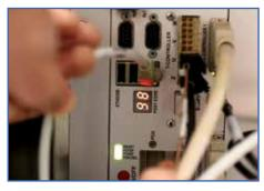
Switch on the top unit. Give it time to display green control lights and the permanent status code ("98" on IPSO for AVANCEIII console) before continuing with next unit.
