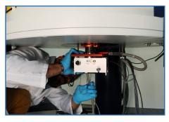
Loosen the screws at the bottom of the probe while holding the probe.
