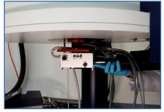
Reinsert the probe and fasten screws. Reconnect all cables and reattach the BCU connection.
