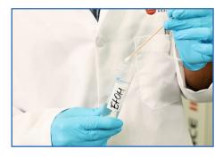
Soak the tip of a cotton swab with 96% ethanol from a clean tube. Use lint-free swabs to ensure probe is not contaminated.
