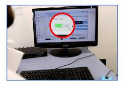
Turn off the temperature control unit (vtu) in TopSpin.
