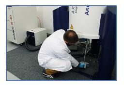
Slide the probe carefully out of the magnet.
