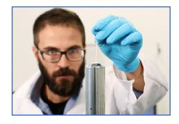
Insert the cotton swab carefully into the upper part of the probe until you feel resistance. Repeat this procedure 2x with fresh, clean ethanol soaked cotton swabs. Let the probe dry for several minutes before remounting.
