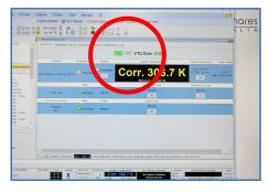
Turn on the temperature control unit (vtu) and wait for 30 minutes. Perform a temperature calibration. (see NMR Maintenance Guide for AXINON® test systems).
