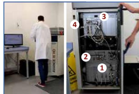
Open the NMR console. Switch off all units from bottom to top (1-3). Give each unit time to shut down completely to avoid any system errors. Then turn off the console power (4).
