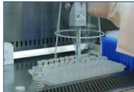
*Place respective additives solution into the prepared sample vials.*
