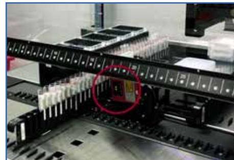
*Sample IDs are automatically scanned by a barcode reader.*
