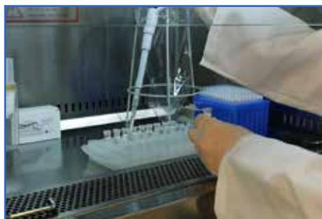
*Transfer the analyte samples to the sample tubes containing the additives solution.*
