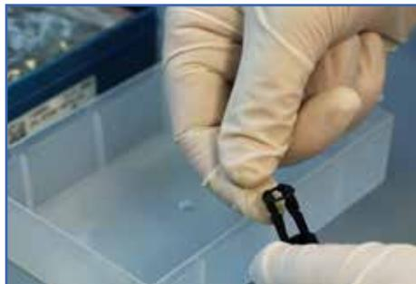
Prepare a new pincer by pulling the o-ring over the pincer's sleeves.
