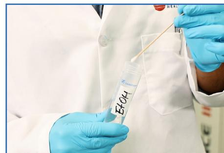
Soak the tip of a cotton swab with 96% ethanol from a clean tube. Use lint-free swabs to ensure probe is not contaminated.
