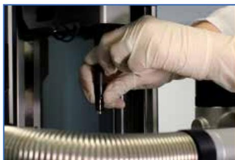
Remove the old pincer by slowly turning while simultaneously pulling it off.
