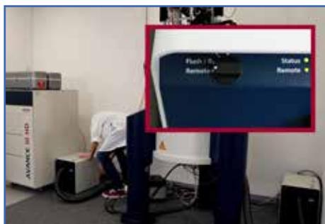
Turn on all BCUs. Check that the controller is set to "remote" and the remote control light is green. Wait at least for 30 minutes.
