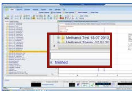
When „ii finished“ appears below the command line, TopSpin is ready for use.
