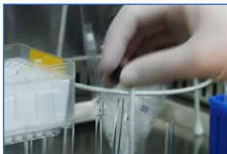
*Close each NMR tube thoroughly with an NMR cap.*
