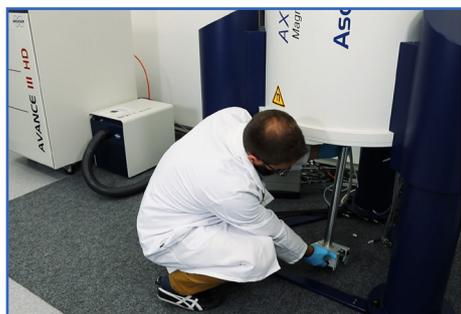
Slide the probe carefully out of the magnet.
