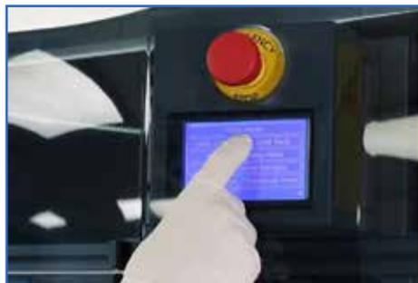
To access the gripper arm in the SampleJet, push "Load rack" and select any rack number of options 1 through 5 on the SampleJet Touch Display.
