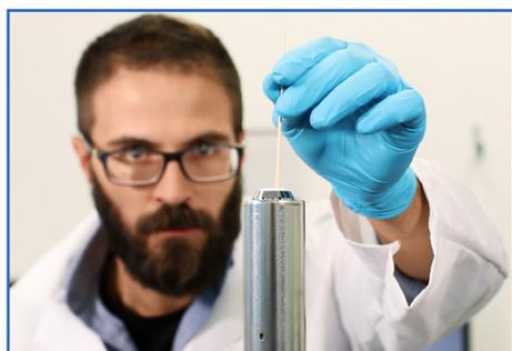
Insert the cotton swab carefully into the upper part of the probe until you feel resistance. Repeat this procedure 2x with fresh, clean ethanol soaked cotton swabs. Let the probe dry for several minutes before remounting.
