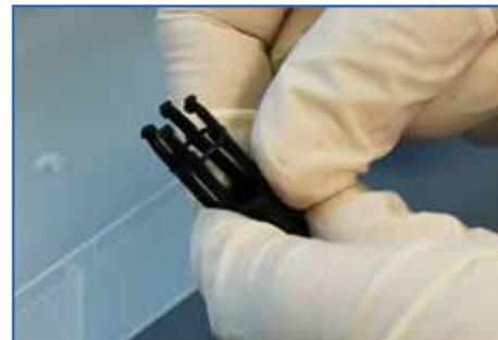
Make sure that the o-ring is placed in the second indentation of the pincer's sleeves.
