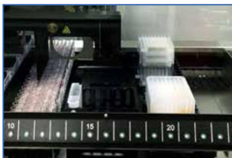
*The analytes are transferred to the 96 well plate containing the additives solution.*
