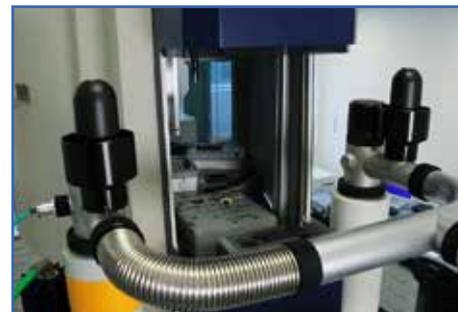
To access the gripper arm, ensure the cover of the SampleJet is pushed upwards.
