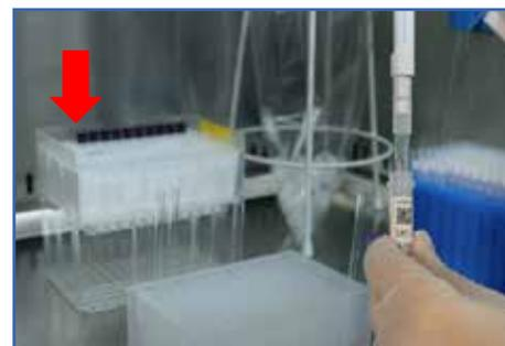
*Prepare 1 NMR tube with calibrator and place at position A1.*
