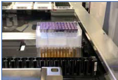
NMR tubes are closed with barcode caps and scanned. The cap barcodes are automatically assigned to the sample ID. The data is captured by the LI(M)S.
