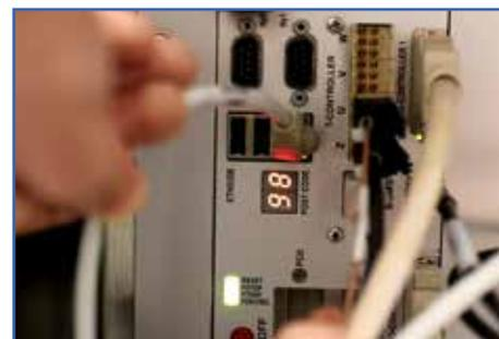
Switch on the top unit. Give it time to display green control lights and the permanent status code („98“ on IPSO for AVANCEIII console) before continuing with next unit.
