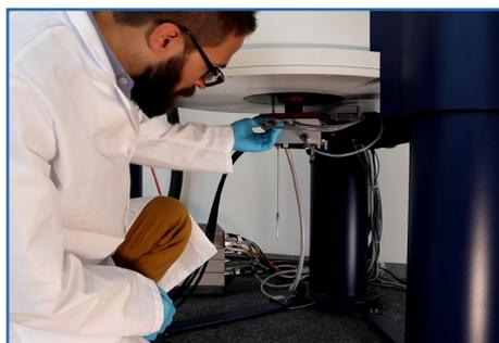
Carefully disconnect all cables and the BCU connection from the probe.
