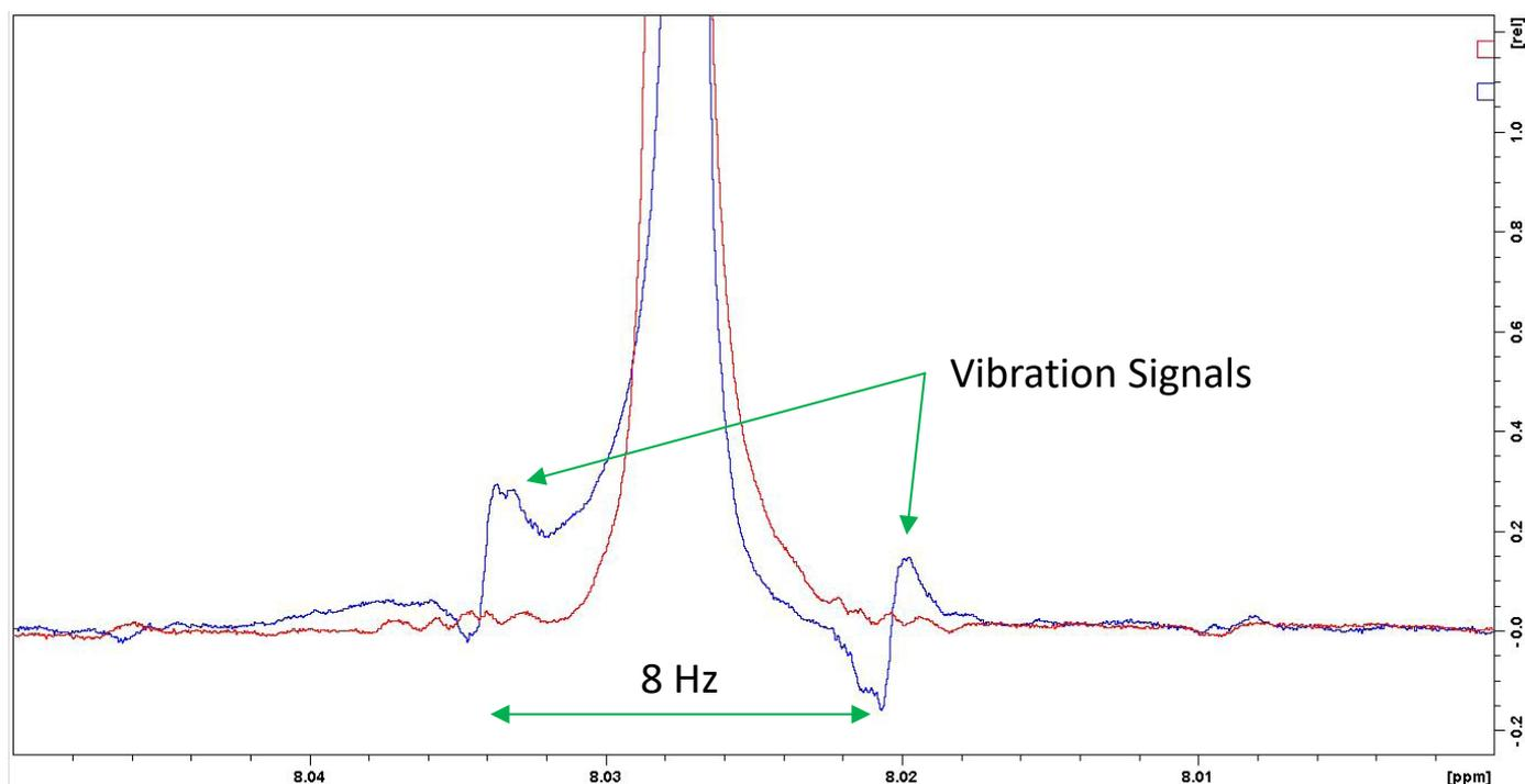
Figure 1: Overlay of a maintenance spectrum with vibrations (blue) and without (red) vibrations. The vibrations can be seen as peaks at +/- 4 Hz around the main signal.
