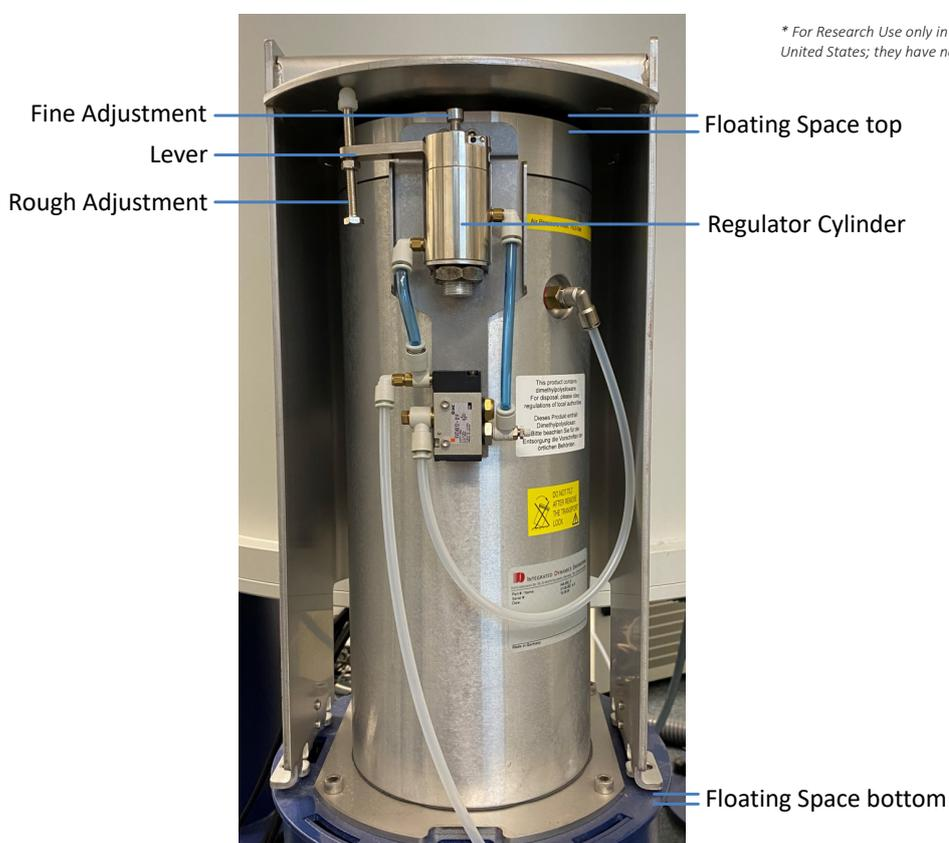
Figure 2: A look behind the cover of the magnet stand: The piston should be float freely above the blue magnet stand at the bottom and above the inner cylinder at the top. Right: Schematic drawing of a damper.
