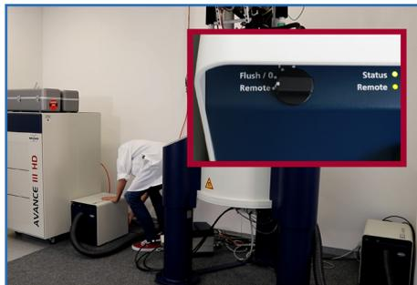
Turn on all BCUs. Check that the controller is set to "remote" and the remote control light is green. Wait at least for 30 minutes.
