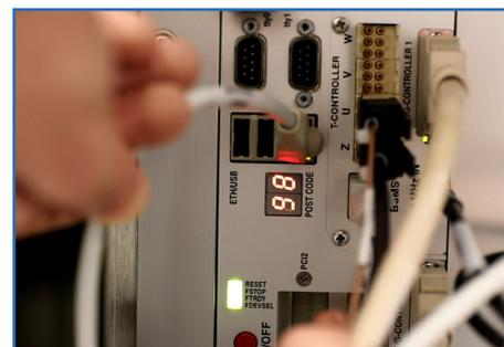
Switch on the top unit. Give it time to display green control lights and the permanent status code („98“ on IPSO for AVANCEIII console) before continuing with next unit.
